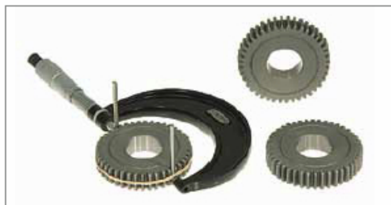
Illustration of gears measured over pins
