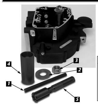
INNER CAM BEARING PULLER USE ON 2006 TO PRESENT FXD Designed like our popular EVO cam bearing tool, it removes the bearing easily without any damage to the crankcase. This precision built tool will also keep the pin rollers from accidentally falling into the crankcase.
