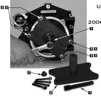
ENGINE CASE SPLITTER USE ON 2007-PRESENT FL'S & FXST'S. USE ON 2006-PRESENT DYNA. USE ON JIMS 120" ENGINE ON 2006 TO PRESENT DYNA & 2007 FL'S, FXST.
