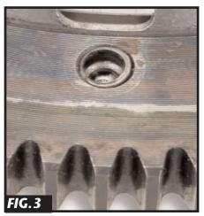
3) Chuck tool drill bit No.2223 into a hand drill, or drill press. Apply a small amount of cutting oil (a little engine oil is ok) then drill rivet at about 300 rpm. **See Fig 5.**
